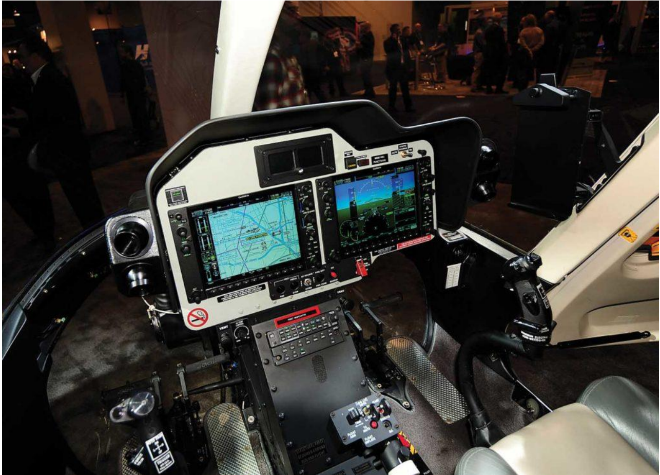
The cockpit of the Bell 407GX i equipped for IFR operations. Skip Robinson Photo
